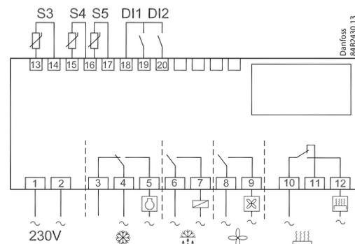
Connection options for EKC 302D (DIN rail model)
