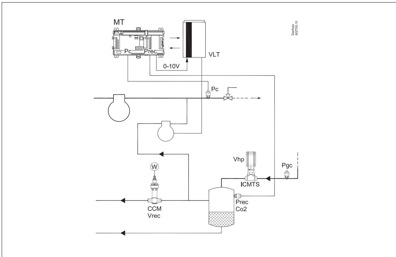
The frequency converter is suitable for controlling a compressor used for parallel compression.
