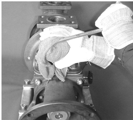
1. Carefully open the oil filler plug (57) ¼ turn and wait until the oil chamber is depressurized (this may take a while!) Use a wet cloth to protect the plug.
