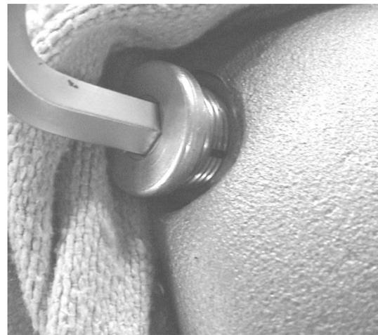
2. The oil fill plug (57) is slotted to avoid a sudden escape of refrigerant. Never use a power tool to open the plug!
