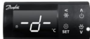
DEFROST: press for 3 seconds to stop manual defrost.
