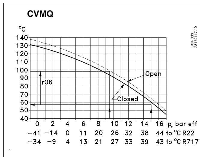
The two curves are shown with the valve's spring setting equaling the factory setting. If the spring setting is changed to a higher pressure, the curve will be displaced correspondingly to a higher temperature.
