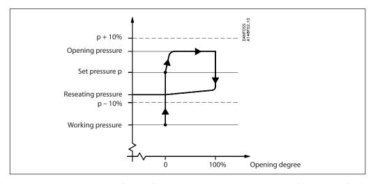
BSV is designed as a standard safety relief valve (DIN 3320) which are recommended for refrigeration plants. On a rise in pressure above the set pressure, the safety relief valve will initially start opening slightly, to minimise the outlet of refrigerant. If the pressure continues to increase, the valve will open fully. The safety relief valve will be fully open before the pressure is 10%
