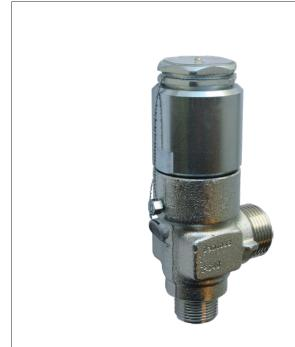
BSV is a standard, back pressure **independent** safety relief valve, especially designed for protection of small components against excessive pressure and as a pilot valve for the pilot operated internal safety valve, type POV.
