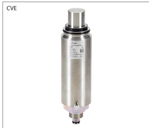
CVE is, when fitted with the ICAD 1200A stepper-motor, a constant pressure pilot valve with electronic change of set-point for a max. working pressure (MWP) of 52 bar (754 psi) and with electronic controlled full range settings of -0.66 to 8 bar gauge (19.5 in. Hg to 116 psi). The CVE interface to the ICAD is hermetic closed and rotation force is transferred from the ICAD by magnetic forces.
