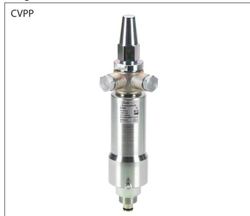
CVPP is a differential-pressure pilot valve for a max. working pressure (MWP) of 52 bar (754 psi) and with 2 setting ranges covering settings of -0.66 to 28 bar (19.5 in. Hg to 406 psi).
