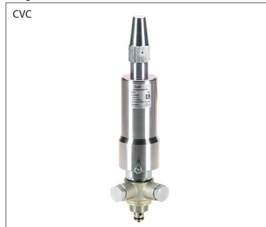
CVC is a constant pressure pilot valve at an external reference point for a max. working pressure (MWP) of 52 bar (754 psi) and with 2 setting ranges covering settings of -0.66 to 28 bar (19.5 in. Hg to 406 psi).
