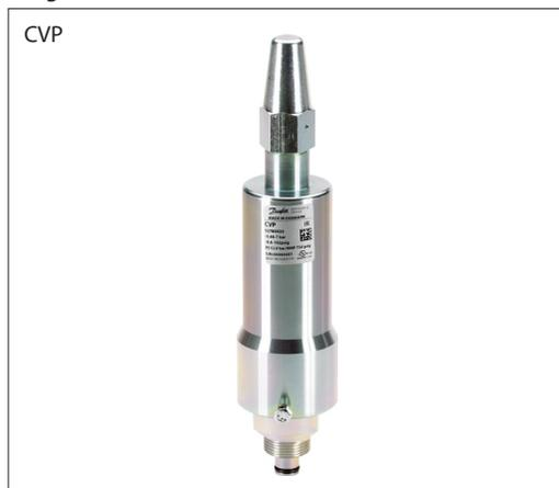
CVP is a constant-pressure pilot valve for a max. working pressure (MWP) of 52 bar (754 psi) and with 3 setting ranges covering settings of -0.66 to 52 bar (19.5 in. Hg to 754 psi).
